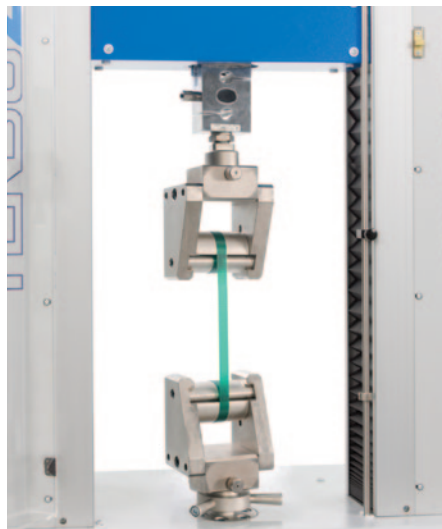
Self-tightening high tenacity clamps for ribbons 100mm wide, Code 2510.920 (for Tenso-Lab 1000-5000 only)
