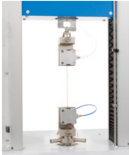
Pneumatic clamps for standard yarns and sewing threads (50N maximum capacity), Code 2510.982
