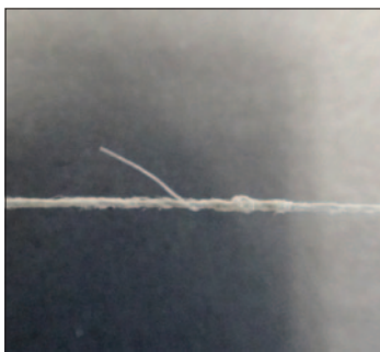
Lycra core protrusion
