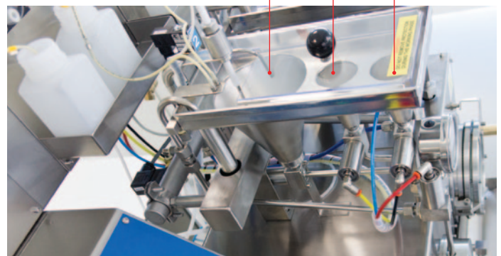
Picture showing the 3 automatic dosing tanks.
