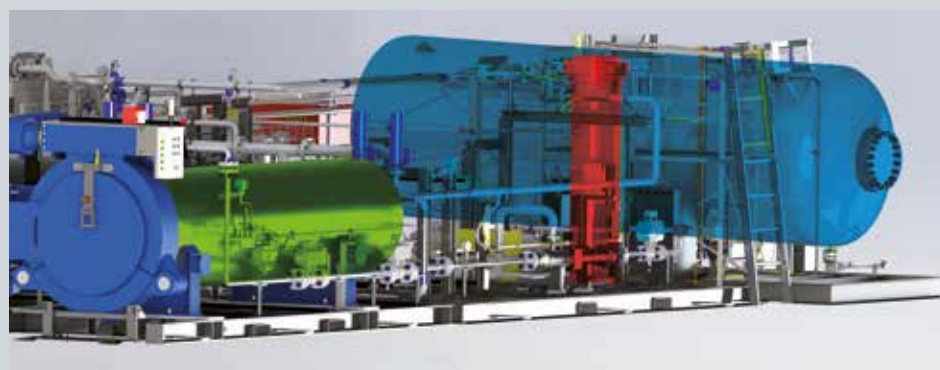
Colours represent the different phases of CO 2 , as represented in the phase diagram.
