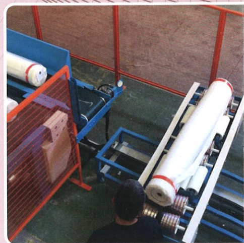
Scarico automatico anima cart Automatic releasing of paper c
